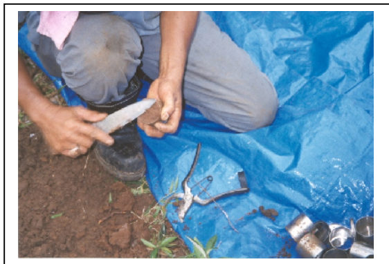
Figure 6. Disposal of the remaining soil from the ring soil sampler (Source photo: JICA, 2002)
